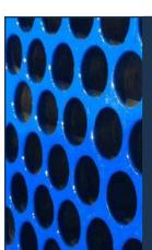
Tubesheet restoration complete using Curran International's polymeric ероху cladding system.
